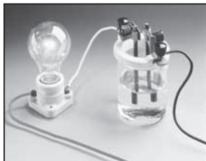
However, the solution of salt water does conduct an electric current, so the bulb lights up.
