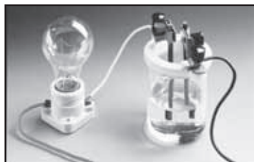
A solution of sugar, a covalent compound, in water does not conduct an electric current. This is because no ions form.
