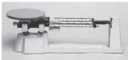
A **balance** is a tool that is used to measure mass.
